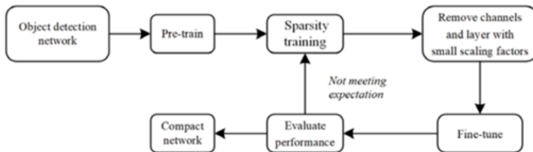
Fig 1: The procedure of a detection model being sparse trained and pruned to a compact model.
