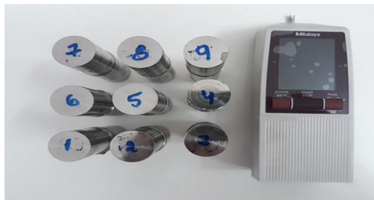
Figure 2. Machined samples & surface roughness tester
