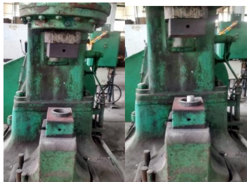
Figure 5: Ring stopper and loading of work piece
