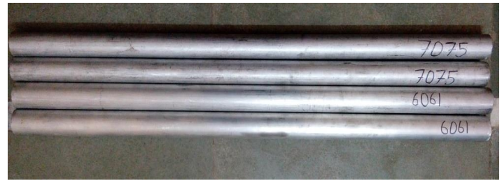
Figure 2: Aluminium alloys 7075 and 6061 specimens.
