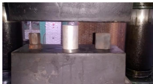
Figure 6: Work Piece material with stoppers in hydraulic Press
