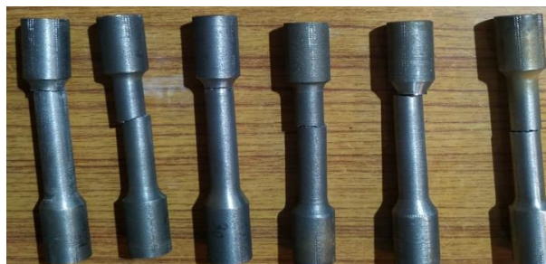
Figure 6. Tensile bar after tensile testing procedure
