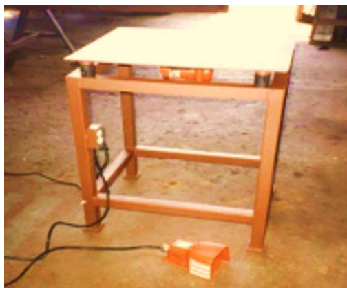
Figure 1. Vibrating table and cast mould experimental setup
