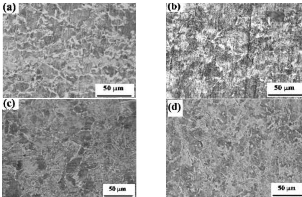
**Fig. 7.** (a) Pearlite – 70% and Ferrite – 30%; (b) Pearlite – 40% and Ferrite – 60%; (c) Pearlite – 25% and Ferrite – 75%; (d) Pearlite – 65% and Ferrite – 35%.
