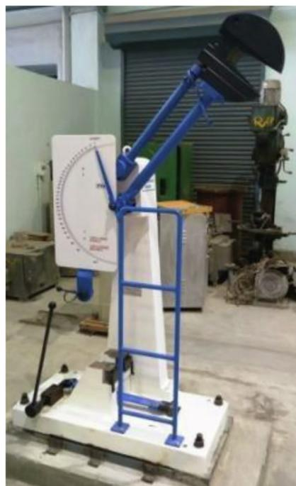
Fig. 5. V-Notch cutting machine and Charpy impact testing machine [13].
