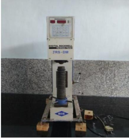
Fig. 4. Digital rockwell hardness testing machine.
