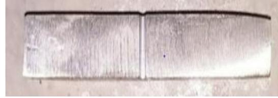
Fig. 6. V-Notch impact testing specimen.
