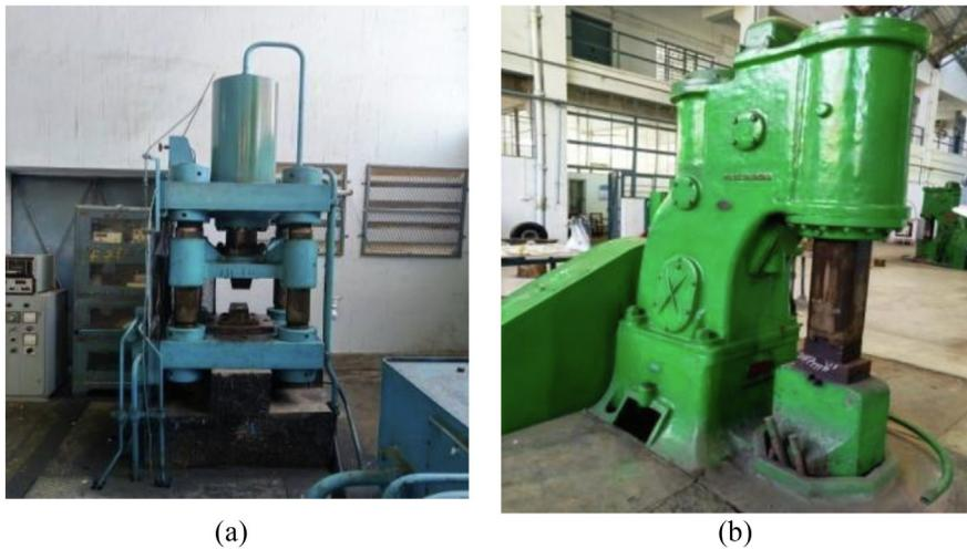
**Fig. 3.** (a) Hydraulic press; (b) Pneumatic Hammer (3cwt).
