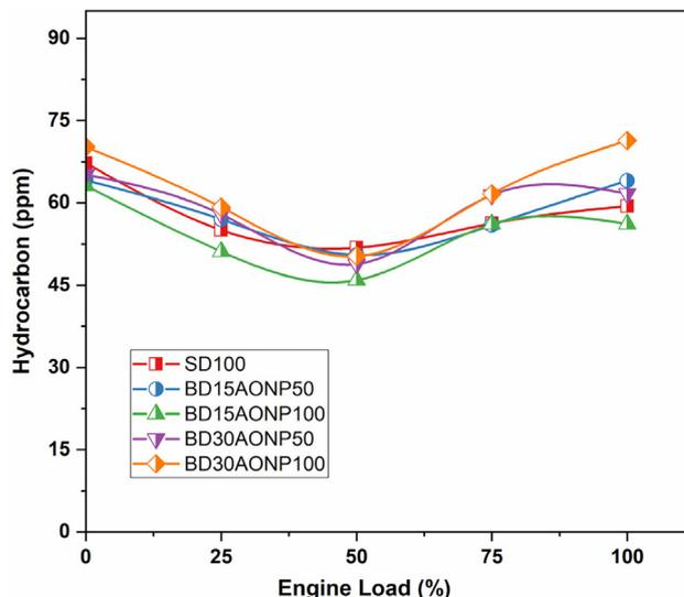
Fig. 5. Effect of AONP on hydrocarbon emission.
