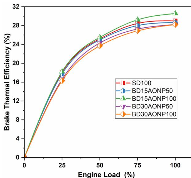
Fig. 2. Effect of AONP on brake thermal efficiency.
