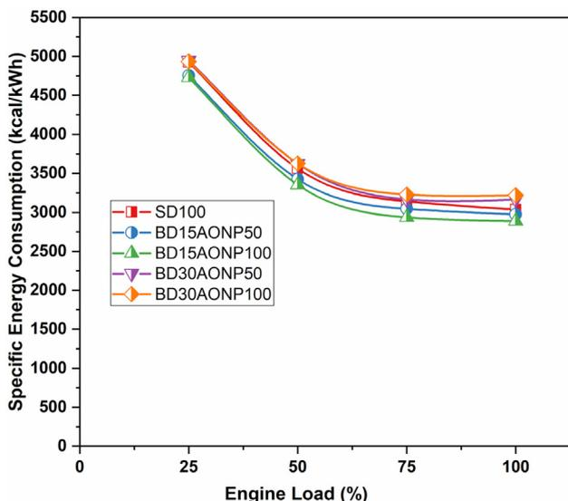
Fig. 3. Effect of AONP on fuel energy consumption.
