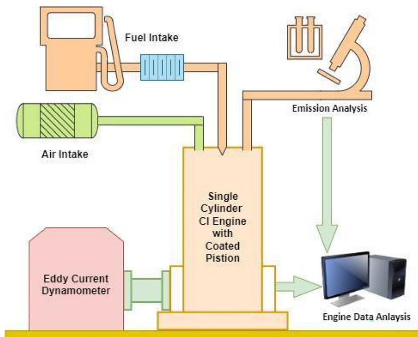
Fig. 1. Experimental engine setup.
