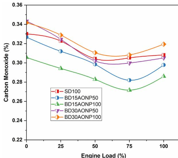
Fig. 4. Effect of AONP on carbon monoxide emission.
