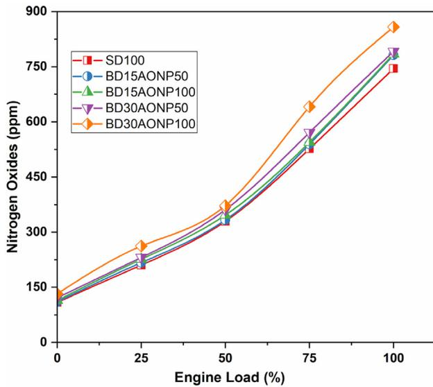
Fig. 6. Effect of AONP on nitrogen oxides emission.
