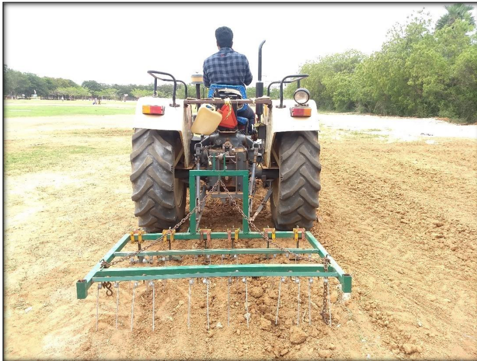
Figure 6: Testing the Multi stage weeder at field conditions.
