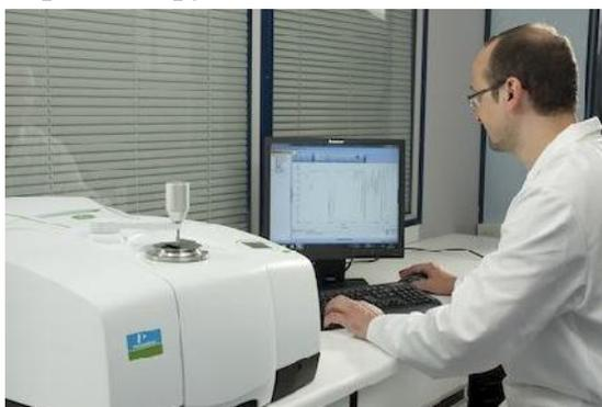
**Figure 5: Perkin Elmer Frontier Fourier Infra-red spectrometer**
