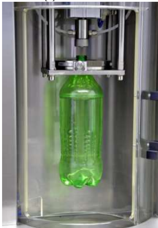
Figure 8: Internal pressure resistance testing
