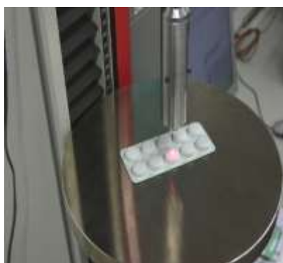
Figure 15: Push out test on blister packing
