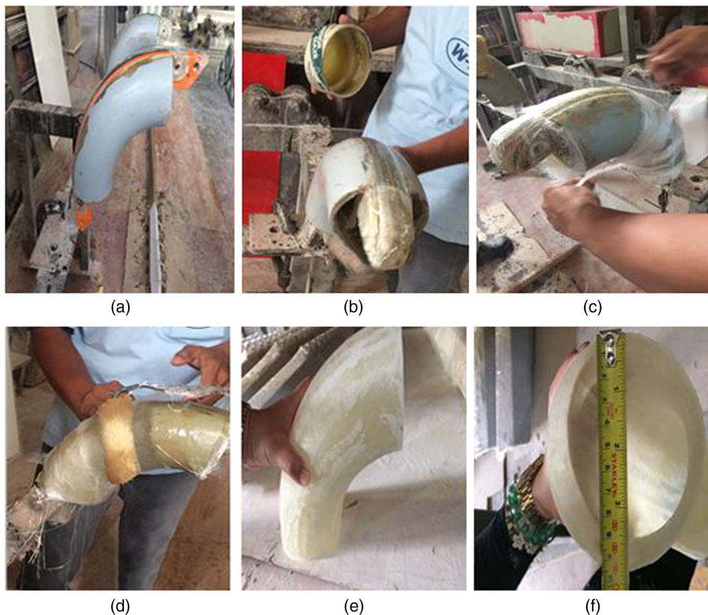
Fig. 1. Fabrication process of E-glass and S-glass elbow joint: (a) mold preparation; (b) applying wax; (c) applying S- and E-mats around the mold; (d) applying resin; (e) completion; and (f) measurement.
