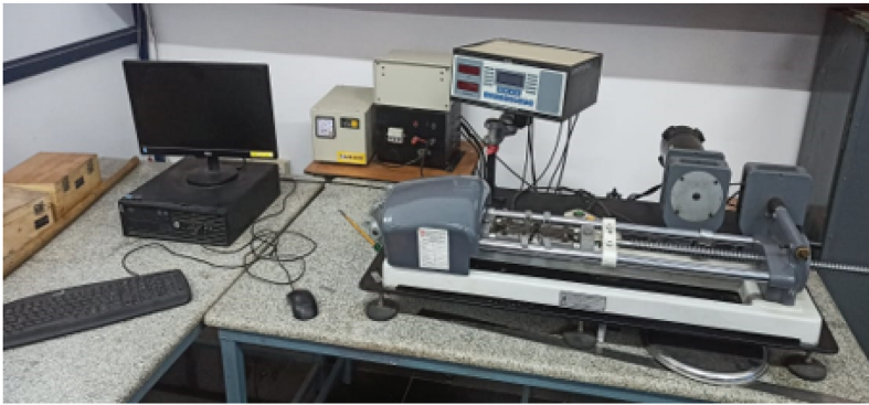
Figure 3. Electronic tensiometer setup for experimental tests .
