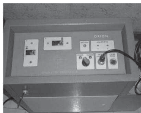
Figure 2.2: Display of instrument showing alignment along x axis (top side) and y axis (left side)
