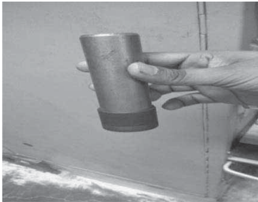
Figure 2.3 b) Gauge used for manual centring
