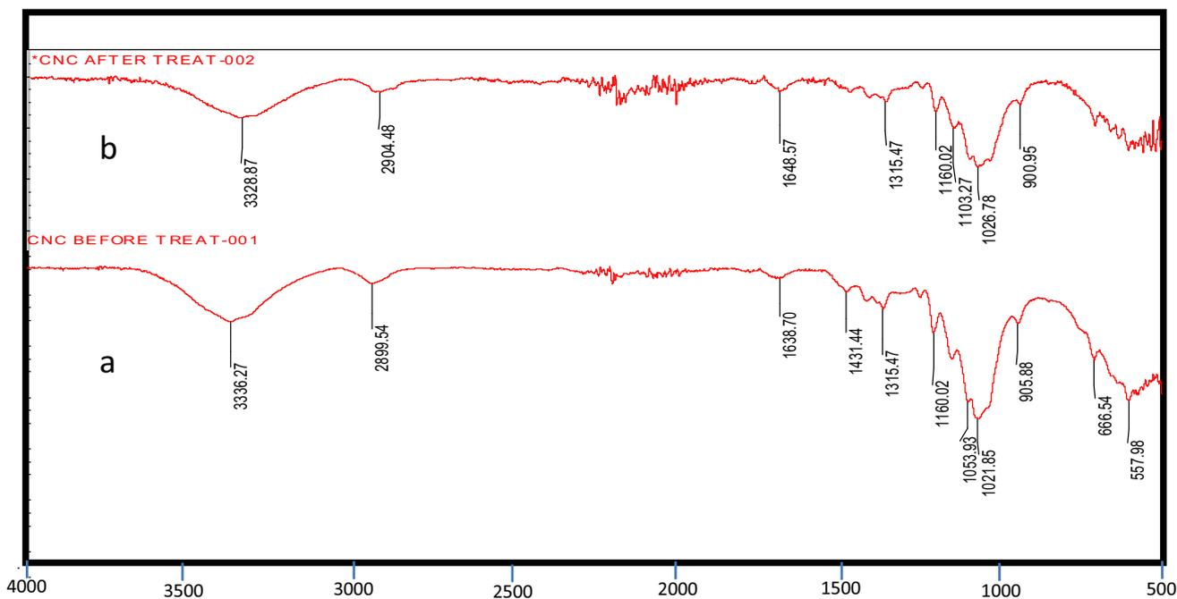
**Fig. 5** FTIR of CNC **a** before adsorption and **b** after adsorption
