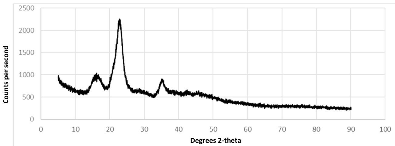
Fig. 8 XRD graph for cellulose nanocrystals
