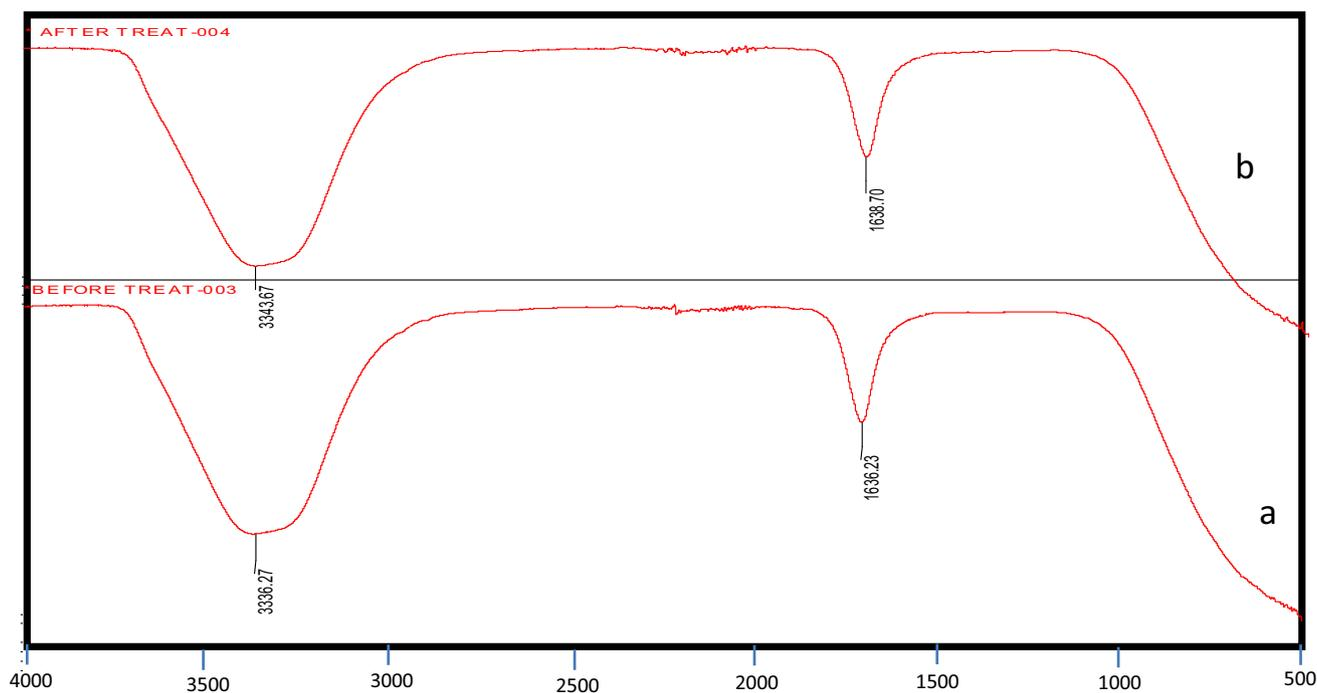
Fig. 6 FTIR of MB dye solution **a** before adsorption and **b** after adsorption
