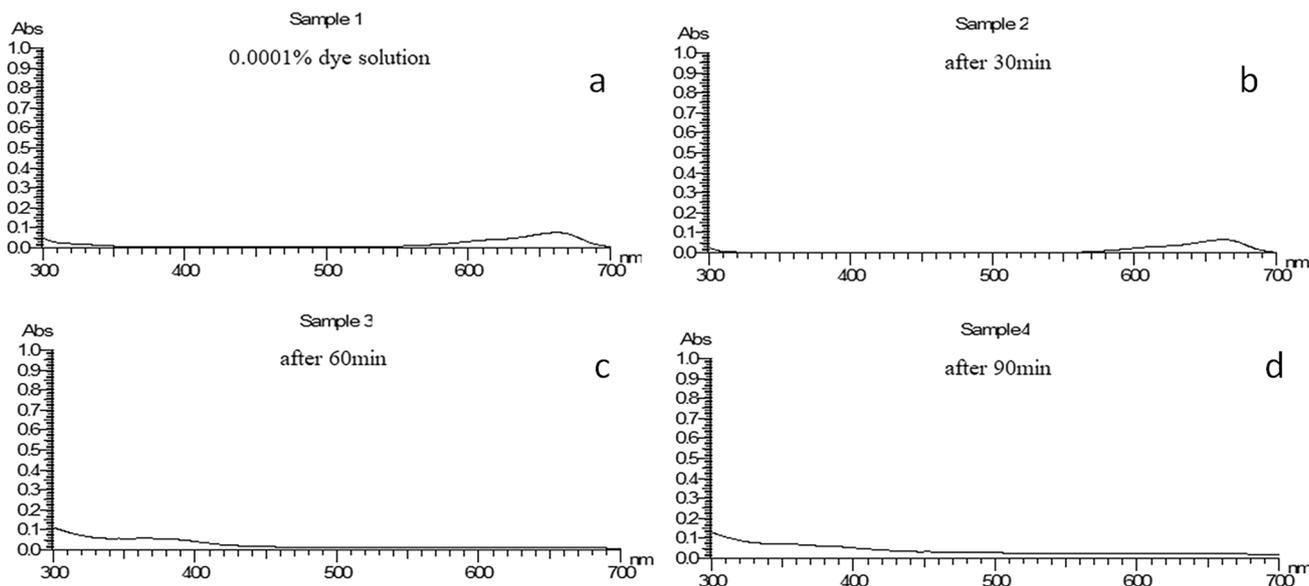
Fig. 9 Absorbency curve of CNC at the different time durations: a stock solution, b 30 min, c 60 min, d 90 min
