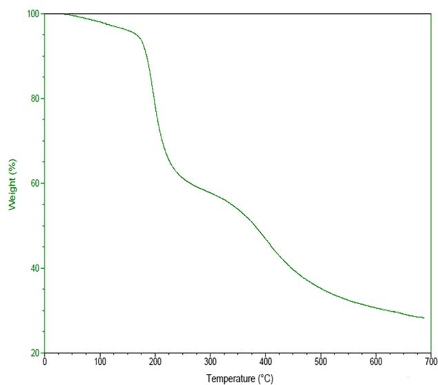
Fig. 7 Thermogravimetric analysis of CNC
