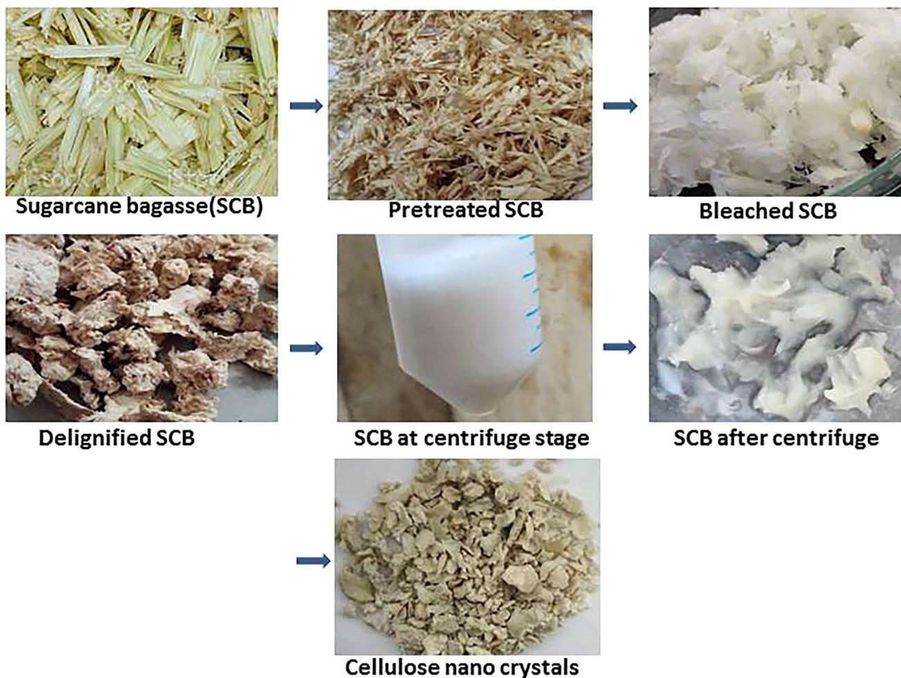
**Fig. 2** Production stages of cellulose nanocrystals from sugarcane bagasse
